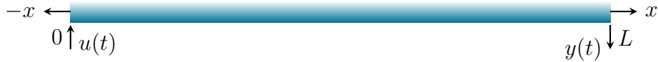
Figure 1.1: A one dimensional rod \Omega of length L with the input source on left side and output source on the right side.
