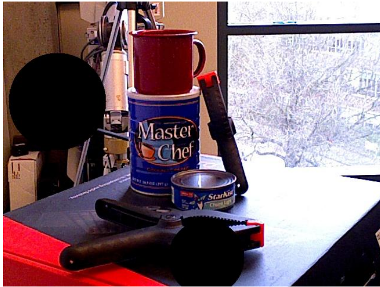
Figure 4.3: An example of an RGB image with the disturbance of missing circles applied at an intensity of two.
